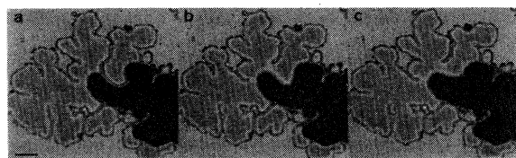
FIG. 6. EggPC vesicle spreading on avidin surface. The dark regions in this figure indicate the adhesion of the upper membrane to the lower, already adhered one. This adhesion mostly follows the existing fjords, but sometimes induces the disappearance of one, as seen in this series of images (arrow) ( \Delta t_{AB} = 0.08 s, \Delta t_{BC} = 1.8 s). The bar is 5 \mu\text{m} long.
